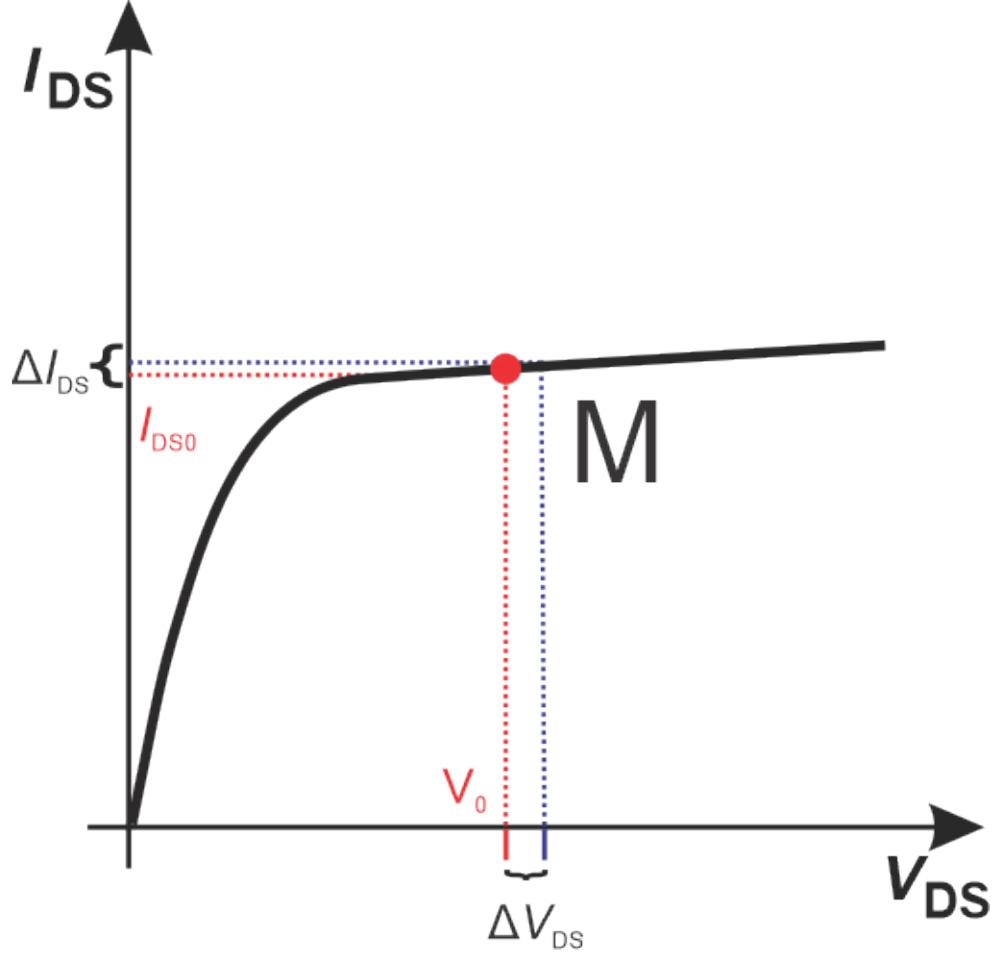
$$I_{DS} = I_{DSS} \cdot \left( \frac{V_{GS}}{V_{TH}} - 1 \right)^2 (1 + \lambda V_{DS})$$
